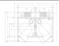
Double Rocky Mountain Double vault. Standard features include 2 ABS lined concrete vaults, board and batt upper and rock lower textured walls, cedar shake textured roof, offloaded and set up at site.
