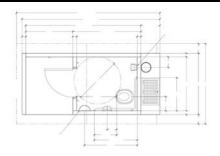
Cascadian Single vault. Standard features include ABS lined concrete vault, board and batt upper and lap siding lower textured walls, cedar shake textured roof, offloaded and set up at site.
