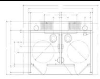
Double Cascadian Double vault. Standard features include 2 ABS lined concrete vaults, board and batt upper and lap siding lower textured walls, cedar shake textured roof, offloaded and set up at site.
