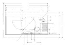
Rocky Mountain Single vault. Standard features include ABS lined concrete vault, board and batt upper and rock lower textured walls, cedar shake textured roof, offloaded and set up at site.
